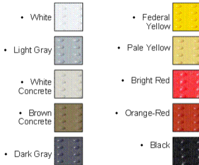
Figure 1. Photographic samples of the 10 single-color detectable warnings tested in the FHWA study
