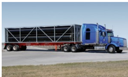
Lincoln Titan modules transport natural gas where infrastructure does not reach.
